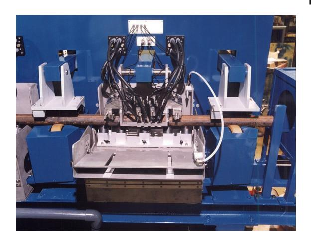
The purpose of this equipment is to provide both ultrasonic and eddy current inspection of tube and bar products. The ultrasonic inspection is achieved using a number of adjustable Water Column Coupled Probe (WCCP) units for shear wave longitudinal flaw detection and fixed WCCP unit for thickness monitoring. The eddy current inspection can be either a rotating eddy current probe or using differential probes mounted in holder. See the reverse of this brochure.
